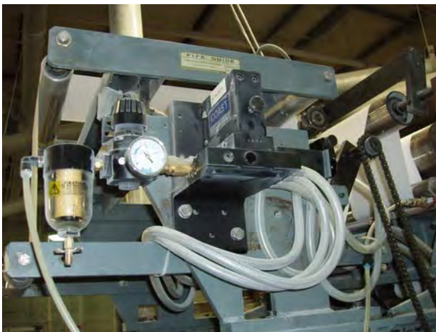
Retrofitting a 17" Fife electrical/mechanical offset pivot guide, on a W&D envelope machine.
