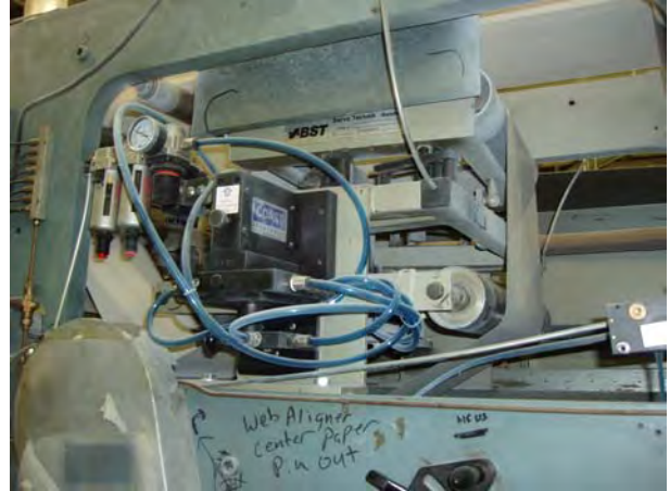
Retrofitting 13" BST, electro/mechanical Displacement Guide on W&D envelope machine.
