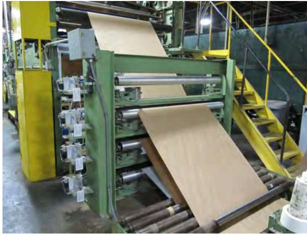
4 Up Steering guide stack, guiding into multi-wall paper bag manufacturing.
