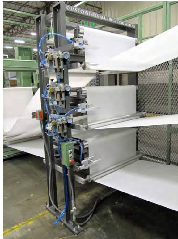
3 Up Displacement guide stack, guiding multiple lines into napkin embossing.
